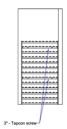
For uneven surfaces, like brick, we recommend using a slotted "L" bracket that you secure to the post with a 5/8" screw and then use a Tapcon screw to secure to the wall.
